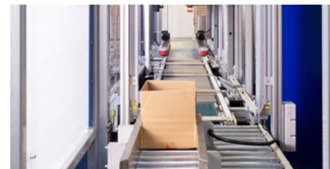
1. DETECTION OF BOX FORMAT AND PRODUCT HEIGHT WITHIN THE BOX
